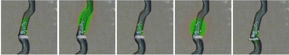
Figure 4.47: Influence of material parameters on sand distribution. From left to right, and top to bottom: reference configuration, low decay, no water transport, high diffusivity, and reversed water flow.
